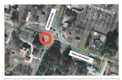
Layout of Roundabout at Pearce's Road/Proctor Street Intersection Installation of a roundabout is projected reduce crashes by 78% according to a 2016 report by Will Letchworth, PE
