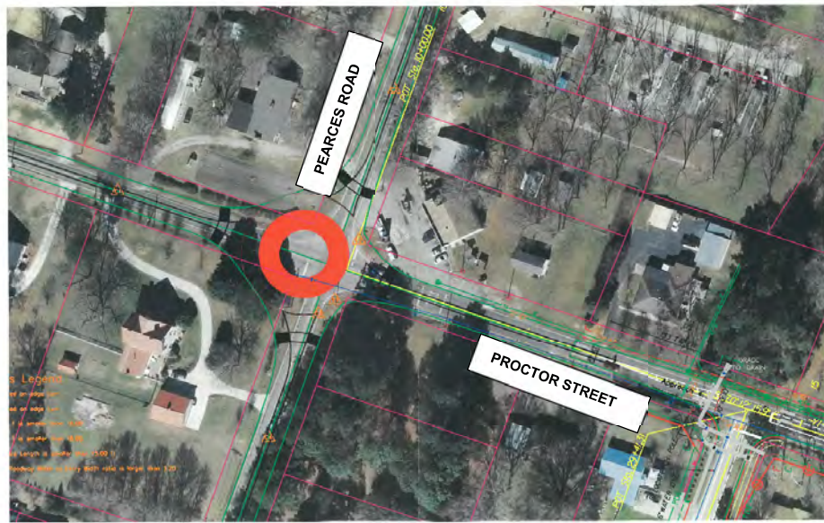
Layout of Roundabout at Pearce's Road/Proctor Street Intersection Installation of a roundabout is projected reduce crashes by
