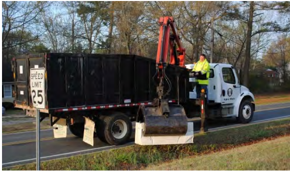
Operator collecting bulk waste with knuckleboom truck
