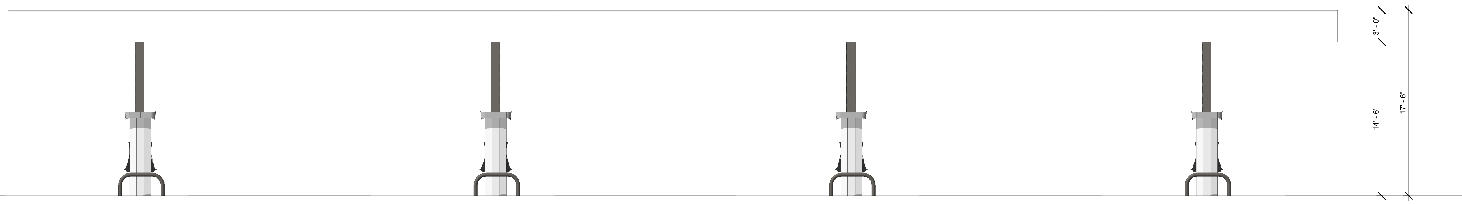
4 FUEL CANOPY LONG ELEVATION - 8 DISPENSERS TOTAL 3/16" = 1'-0"
